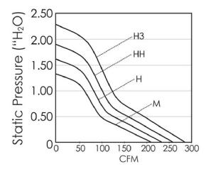
It is essentially a measure of the differential air pressure between the air pressure inside an application vs ambient air pressure outside of an application. There is an inverse relationship between airflow and static pressure. As the pressure differential rises, airflow drops.
