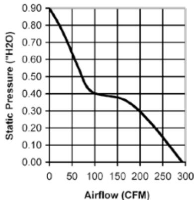
Static Pressure is usually stated either in inches of water (H<sub>2</sub>O) or in millimeters of water (mmH<sub>2</sub>O). It is essentially a measure of the differential air pressure between the air pressures inside an application vs ambient air pressure outside of an application, which for airflow calculation purposes is usually 0 (zero). There is an inverse relationship between airflow and static pressure. As the pressure differential rises, airflow drops.
