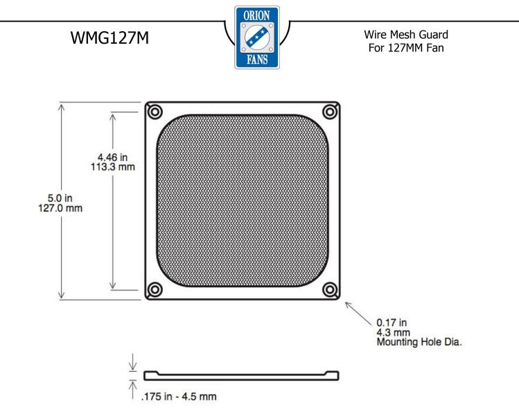
Aluminum Frame / Stainless Steel Mesh filters offer high levels of air passage while efficiently filtering contaminants and shielding from EMI/RFI.
