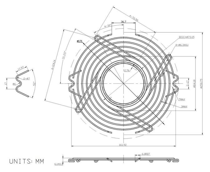
Steel wire guards with Zinc plating offer high levels of air passage while providing protection from injury and intake of solid objects. The Zinc plating ensures years of corrosion-free reliability.
