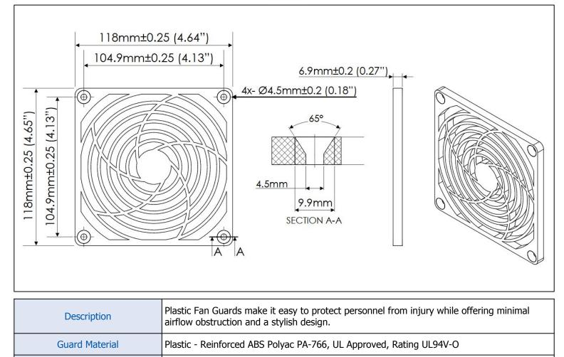
Mounting Ø4.5mm mounting holes, 65° Countersink.
