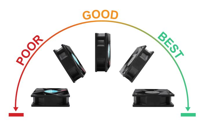
Avoid mounting sealed sleeve bearing fans with the impeller facing down.
